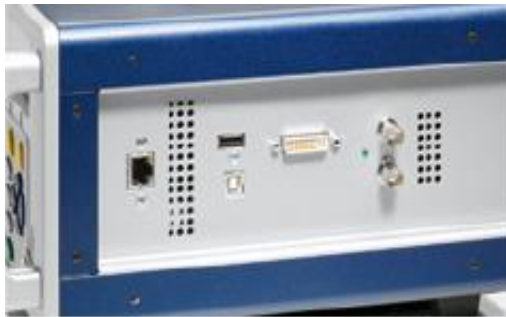
Overview about interfaces: Ethernet, RJ45, ASI In/Out over BNC, USB-A, USB-B, SCART, DIV-out.
